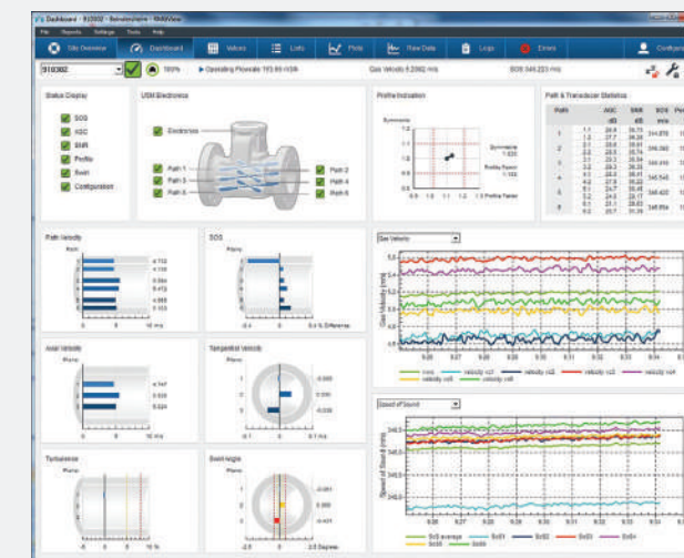
RMGView USM facilitates real-time performance monitoring of CBM parameters
