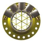
**Q.Sonic-4** - **Exceeding industry standards:** In addition to the 2 double reflection paths of the Q.Sonic-3 the Q.Sonic-4 has 2 single reflection paths crossing each other at an angle of 90°. This makes the meter less sensitive to asymmetric flow distortions and results in a 10D straight upstream requirement. The meter is designed for short upstream lengths which are most common with offshore applications and measurement and regulation stations.
